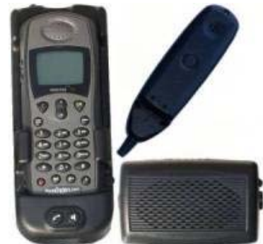
Sattrans Dock for the 9505A
